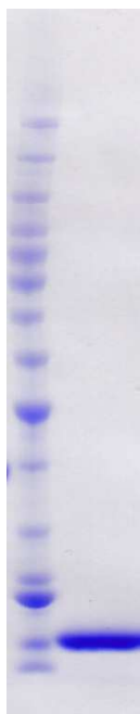
Coomassie blue stained SDS-PAGE (4-12% acrylamide) of 4 \mu\text{g} of RBC BRD3-2 (His). MW markers (left lane) are, from top, 220, 160, 120, 100, 90, 80, 70, 60, 50, 40, 30, 25, 20, 15 & 10 kDa.
