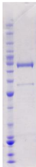
Coomassie blue stained SDS-PAGE (4-12% acrylamide) of 4 μg of purified PRDM9. MW markers at left, are from top: 220, 160, 120, 100, 90, 80, 70, 60, 50, 40, 30, 25, 20, 15, & 10 kDa.
