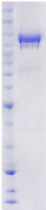
Coomassie blue-stained SDS-PAGE (12% acrylamide) of 5 \mu\text{g} of RBC UHRF1-Full Length (GST). MW markers (left) are, from top, 220, 160, 120, 100, 90, 80, 70, 60, 50 , 40, 30, 25, 20 , 15, 10 kDa.
