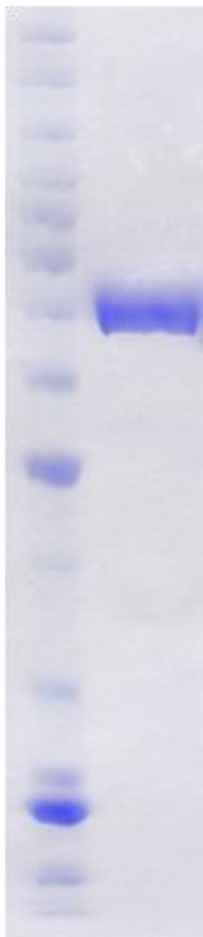
Coomassie blue stained SDS-PAGE (4-20% acrylamide) of 4 \mu g of RBC PAD2. MW markers (left) are, from top, 220, 160, 120, 100, 90, 80, 70, 60, 50, 40, 30, 25, 20, 15, 10 kDa.
