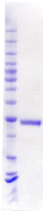
Coomassie blue stained SDS-PAGE (4-12% acrylamide) of 2 μg of purified RBC SMYD3. MW markers (left) are, from top, 220, 160, 120, 90, 70, 60, 50, 40, 30, 25, 20, 15, 10 kDa.
