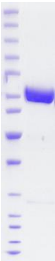
Coomassie blue-stained SDS-PAGE (4-12% acrylamide) of 4 µg of RBC BLM. MW markers (left) are, from top, 200, 150, 120, 100, 85, 70, 60, 50 , 40, 30, 25, 20 , 15, & 10 kDa.
